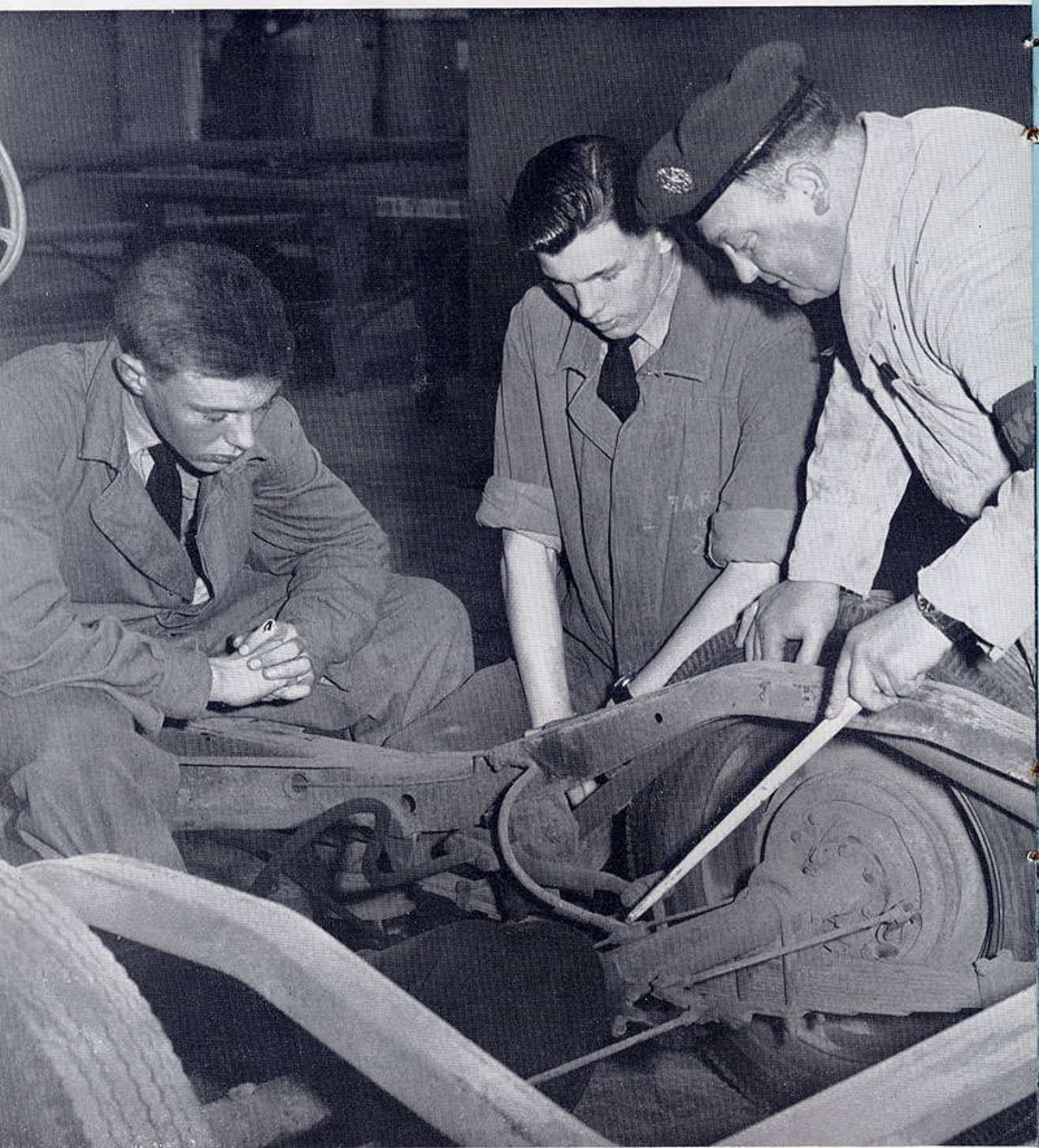
A Flight Sergeant explains the braking system of a Vanguard to boys who are training to be mechanical transport mechanics
